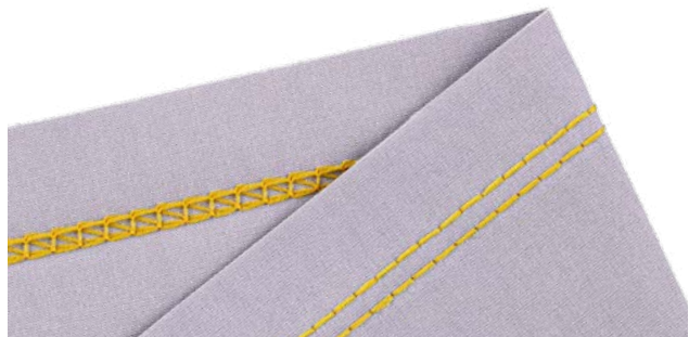
3-thread Cover Stitch narrow (3 mm) for hemming, sewing bindings and decorative effects
